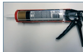
Figure 5. Caulking gun and sealant.
